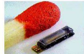
Micro Syringe - attached to intra-vascular endoscope for drug injection
